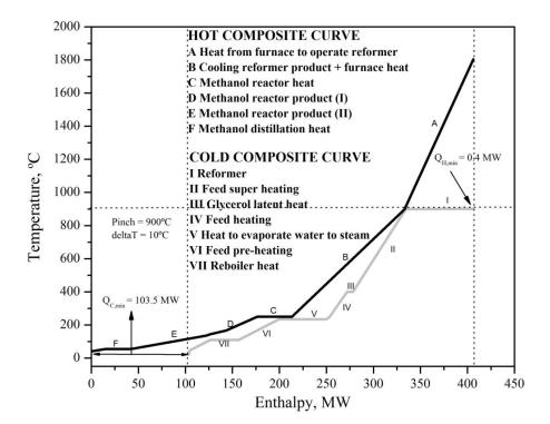
Figure 4: Pinch analysis for (bio)methanol production via hybrid steam reforming of glycerol with methane (Case 6).
