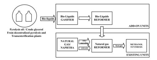
Figure 2: Schematic representation of the HSR concept.
