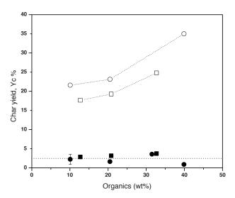
Figure 5: Effect of organics on char yield by different heating rates. reactor temperature =  $510 \pm 10^{\circ}\text{C}$ , -- •-- Glucose atomization, ----- Aqueous fraction atomization, ------ Glucose (glass tube -  $100 \, ^{\circ}\text{C/min}$ ), --  $\Box$ -- Aqueous fraction (glass tube -  $100 \, ^{\circ}\text{C/min}$ ).
