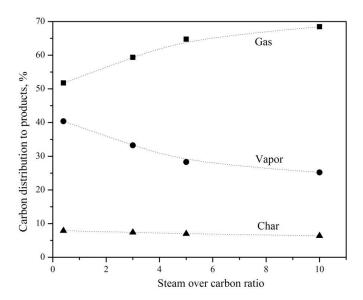
Figure 8: Carbon distribution during gasification of pyrolysis oil, altering the steam-to-carbon ratio (at 800°C).
