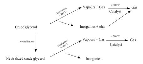
Figure 12: Mechanism of glycerol gasification.
