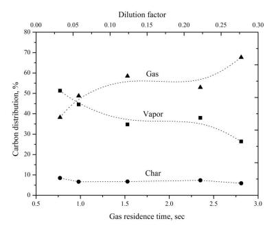
Figure 7: Effect of residence time of gases during gasification of pyrolysis oil, (at  $T=750^{\circ}C$ , S/C=0.4).
