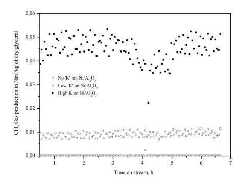
Figure 3: Steam reforming of pure glycerol at T=800°C, S/C=3 using potassium impregnated on Ni/Al $_2$ O $_3$  catalyst. Gas production of methane is presented.
