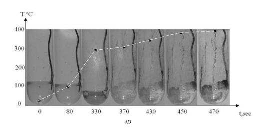
Figure 4: Snapshots of batch tubes during gasification of (a) Glycerol; (b) glycerol with KOH; (c) crude glycerol 1; (d) crude glycerol 2.
