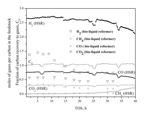
Figure 11: Performance of Catalyst A (Ni/K-Mg-Al $_2O_3$ ) and Catalyst B (Ni/Al $_2O_3$ ) during HSR of methane and crude glycerol. Primary reformer (CH4:crude glycerol= 0.72:0.28 (carbon basis), —  $T_{primary} \sim 820$  °C, S/C $_{primary} \sim 820$  °C, S/C $_{$
