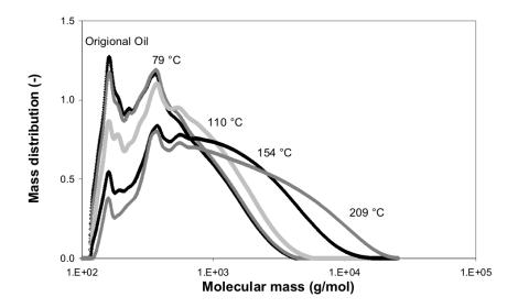
Figure 4: GPC results of the original pyrolysis oil (sample 1) and of residues after heating (samples 2 till 5). The displayed temperatures are of the actual liquid (at 'steady-state').
