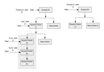
Figure 1: A schematic process diagram of water addition in different amounts to the pyrolysis oil.
