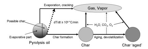
Figure 10: Evaporation scheme of pyrolysis oil leading to gases, vapors and char. The formed char can age to form a less reactive char. Both chars can be converted either by gasification (steam and CO<sub>2</sub>) or combustion. The temperature-time trajectory will determine which pathways are more dominant.
