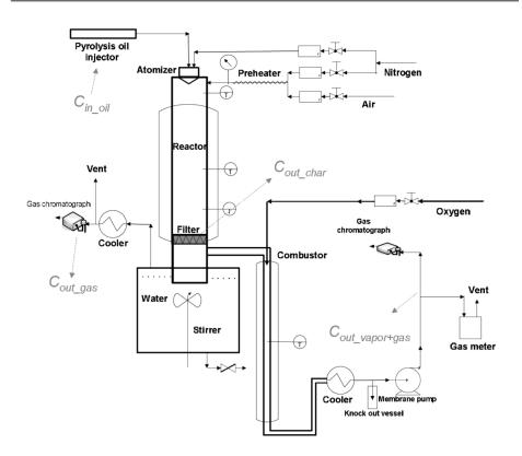
Figure 1: Schematic overview of the continuous pyrolysis evaporation set-up for measuring the carbon distribution from the oil to gas, vapor and char. The amount of gas and char are measured directly, the vapor amount is calculated by difference.
