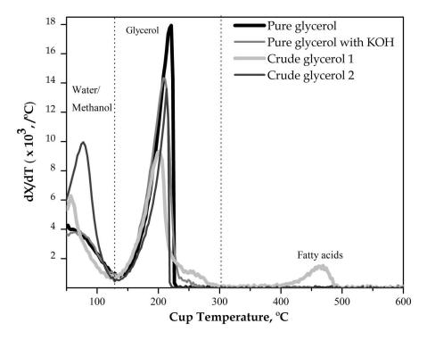
Figure 3: TGA of crude glycerol, pure glycerol with and without KOH at 5  $^{\circ}\text{C/min}$  heating rate in inert  $N_2$  gas.
