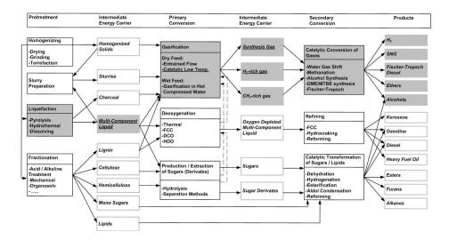
Figure 1: Overview of biomass thermochemical conversion of biomass (adapted from Kersten *et al.* [8]. The highlighted route encompasses pyrolysis oil steam reforming / gasification for the production of synthesis gas: a conversion route investigated in this Thesis.
