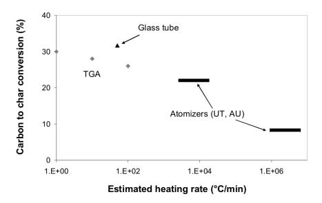
Figure 6: Carbon to char conversion of pyrolysis oil versus estimated heating rates of the following equipment: Thermo-Gravimetric Analysis (TGA), heated glass tube and droplet evaporation using two different atomizer types (UT and UA).
