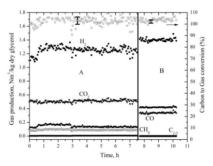
Figure 7: Pre-reforming and steam reforming of glycerol (A) LTR, S/C = 3,  $T_{cat}$  = 588°C and (B) HTR, S/C = 3,  $T_{cat}$  = 787°C. For all cases GC<sub>1</sub>HSV = 838 h<sup>-1</sup>.
