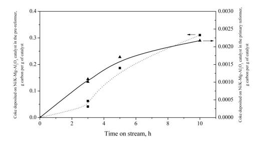
Figure 5: Coke deposition on Ni/K-Mg-Al<sub>2</sub>O<sub>3</sub> catalyst in the bio-liquid reformer (operated at S/C~12,  $T_{bio-liquid\ reformer}$  ~750 °C, CH<sub>4</sub>: pyrolysis oil = 74:26 on carbon weight basis,  $G_{C1}HSV \sim 750\ h^{-1}$ ) and primary reformer (operated at S/C ~3,  $T_{primary}$  = 785 °C,  $G_{C1}HSV \sim 1150\ h^{-1}$ ). The time on stream is of the duration of hybrid steam reforming.
