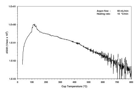
Figure 3: TGA of pyrolysis oil at 10° C/min heating rate in inert (Argon) gas.
