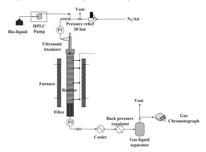
Figure 2: Schematic representation of high pressure gasification of bio-liquids set-up.
