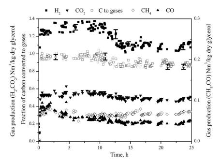
Figure 8: Long duration pre-reforming of glycerol at T = 590°C, S/C = 3.5,  $GC_1HSV = 543 h^{-1}$ .
